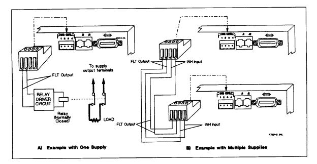
Figure D-3. Examples of FLT Outputs
